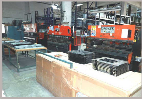
Hydraulic CNC bending machines setup for precise & accurate bending of all sheet metal parts in SS & CRCA steel
