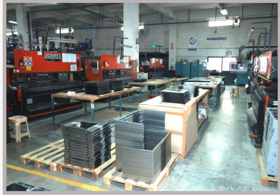
Hydraulic CNC bending machines setup for precise & accurate bending of all sheet metal parts in SS & CRCA steel
